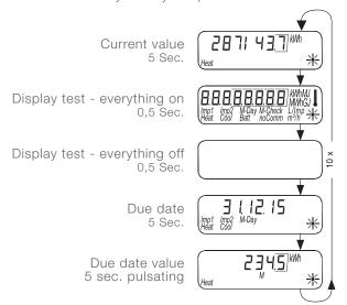
The fast readout display starts with the current consumption value.
